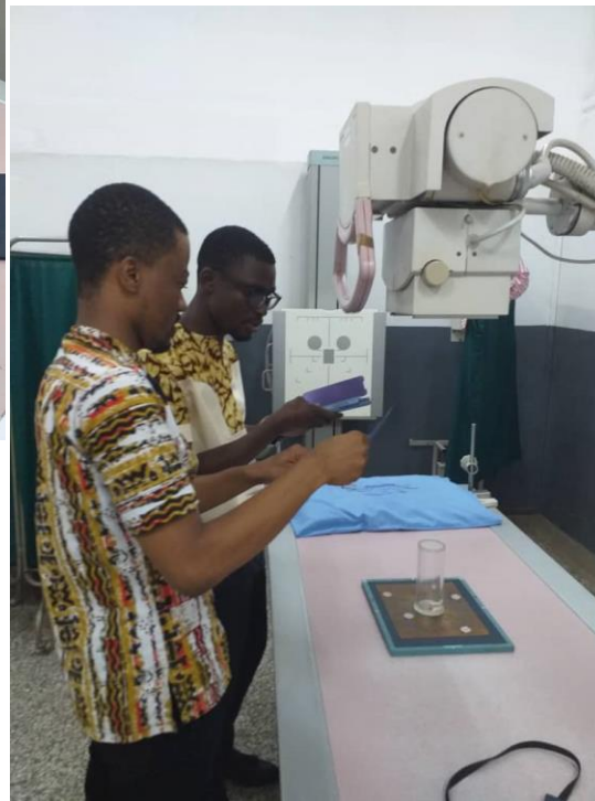
Audit of planar X-ray systems: X-ray field/light alignment
